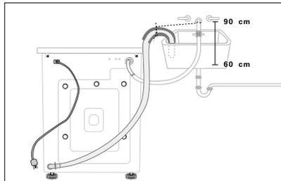
In a sink drain pipe branch
